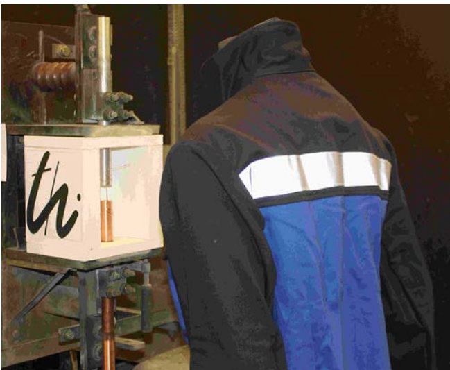
Fig. A 2-1 Test setup, Box test method
