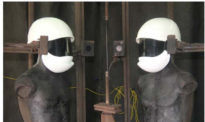
Fig. A 2-2 ATPV Test setup
